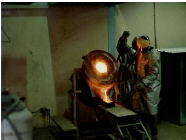
Figure 10.2 – Pouring molten gold
