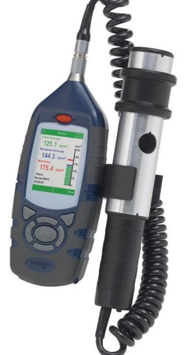
Using a real-time hand-held device enables us to take readings of airborne fumes, at the exhaust outlet.
