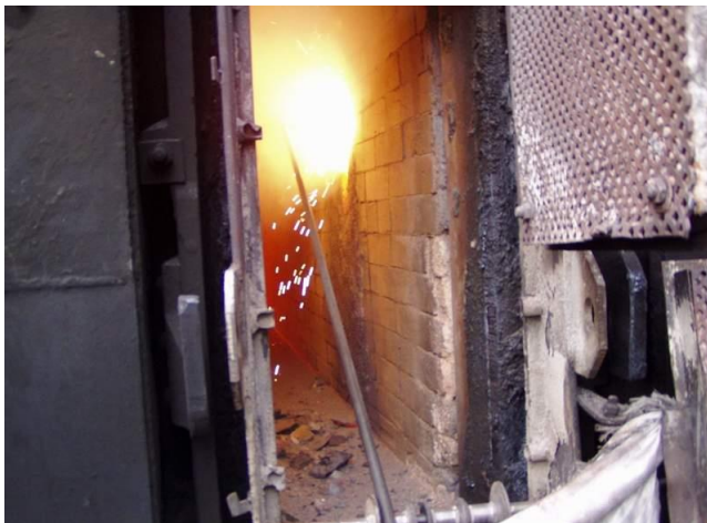
Photograph 5 – Refractory Brick Wall to be Removed
