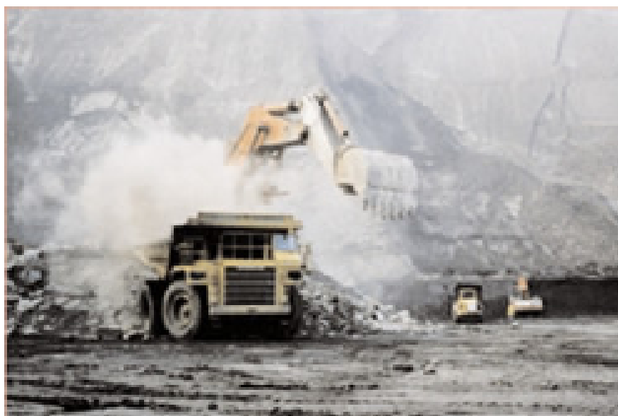
Figure 10.7 – Loading lorry using mechanical arm
