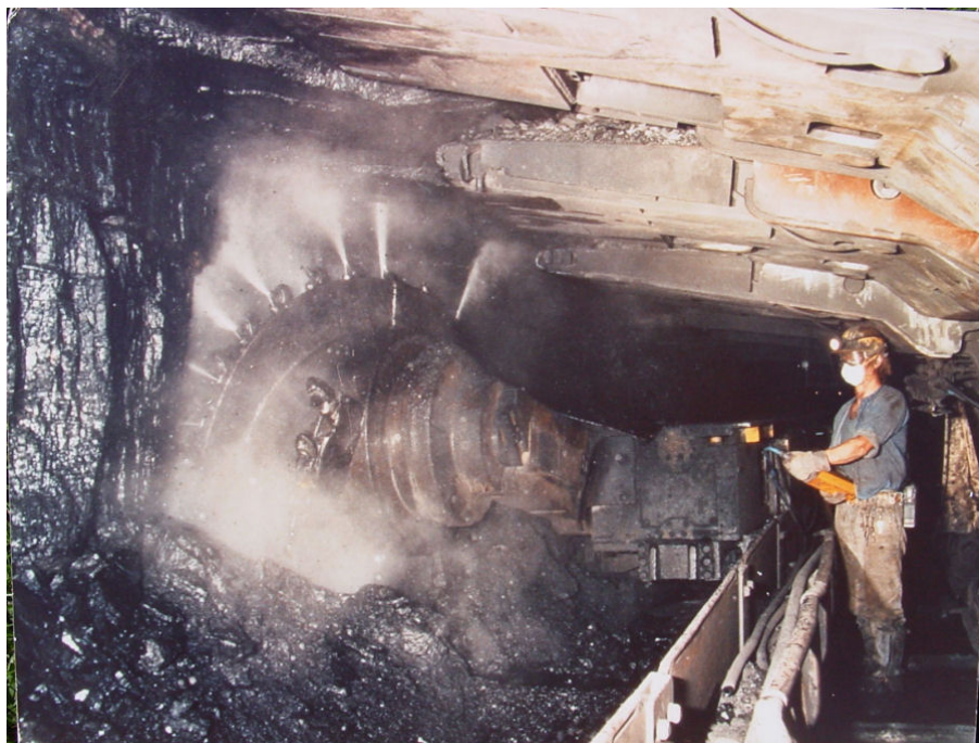
Figure 10.9 – Longwall coal mining with water sprays
