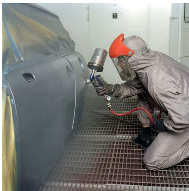
Figure 9.15 – Spraying isocyanate based paint in paint spray booth
