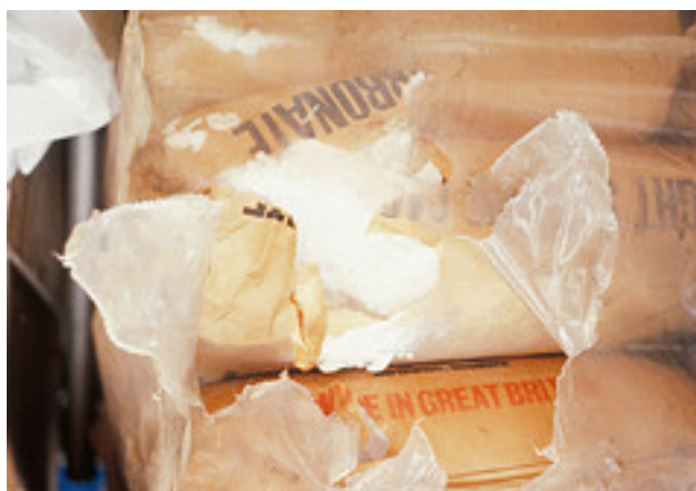
Figure 9.1 – Split bag containing sodium carbonate
