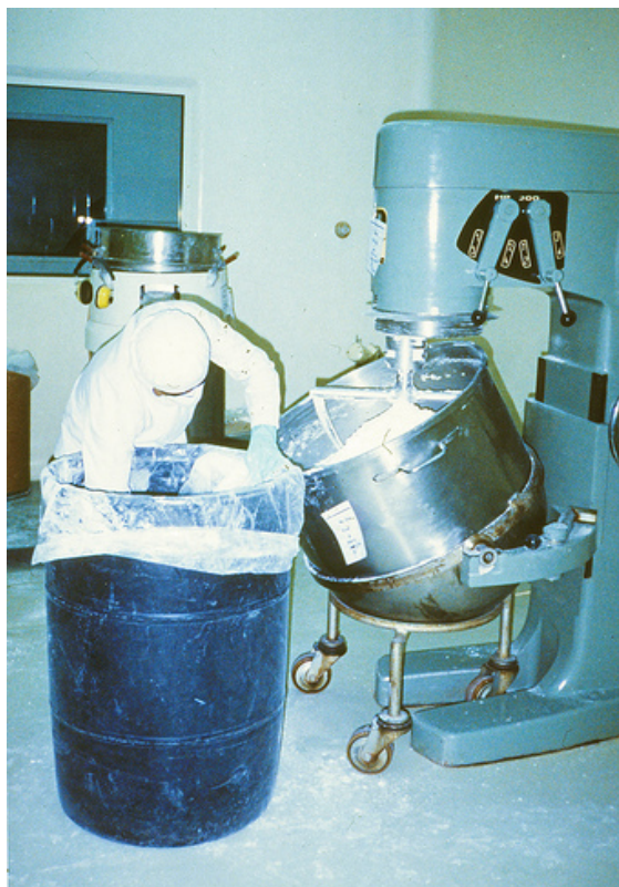
Figure 9.2 – Manual loading of open mixer from drum
