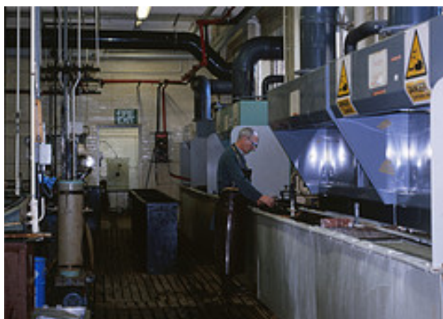
Figure 9.10 – Electroplating bath fitted with local exhaust ventilation
