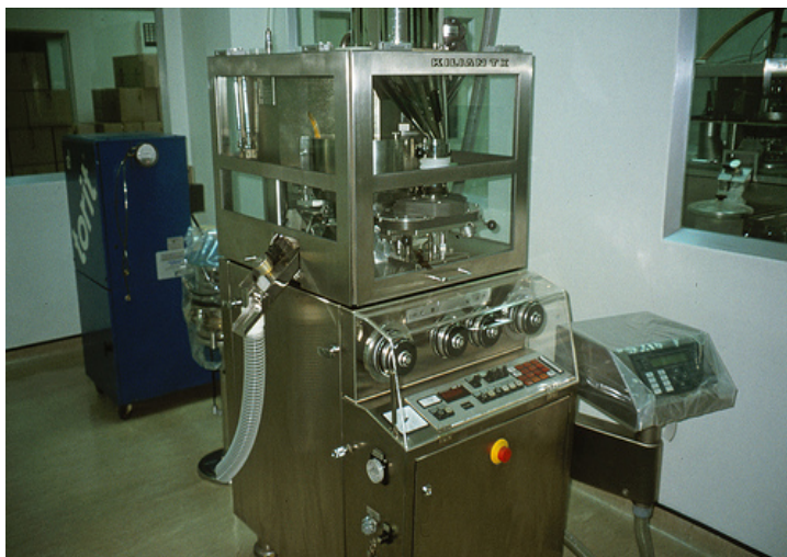
Figure 10.11 – Fully enclosed tablet press with extraction
