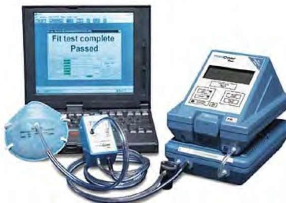
Figure 8.12 – TSI Fit Test Particle Counter
