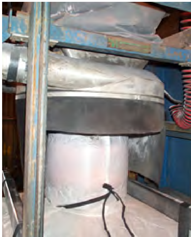
Figure 10.11 – Local Exhaust Ventilation During Bag Filling
