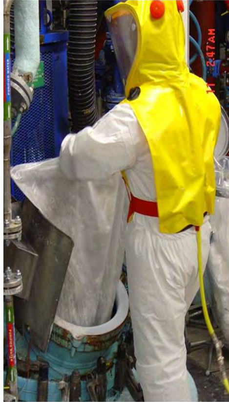
Figure 10.16 – Loading Material into a Dissolving Vessel
