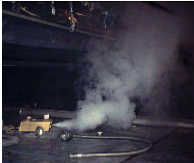
Figure 6.13 - Start of smoke test inside enclosure
