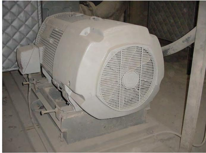
**Figure 4.1 - Totally-enclosed fan cooled electric motor**
