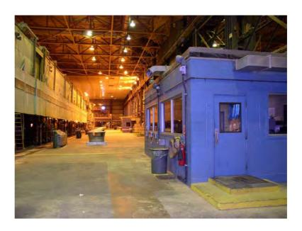
Figure 4.30 - Acoustical control room and noise refuge in a paper manufacturing facility
