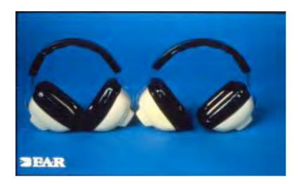
The earmuff head band on the left still maintains its original spring-loaded shape, while the muff on the right shows a head band that has been bent back enough over time to render this device less effective. The earmuff on the right should be discarded.
