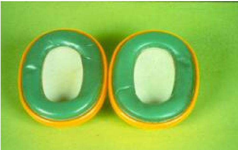
Both earmuff cushions show permanent impressions, which allow air leaks and reduces the attenuation. The cushions need to be replaced.
