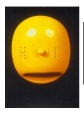
These muffs are the property of H.C. Small holes have been drilled into the earmuff cup to personalize or identify the owner of this device. Unfortunately, attenuation is sacrificed and these muffs need to be removed from service. Be careful to inspect earmuffs for unintentional, and sometimes intentional, modification that can defeat the attenuation.
