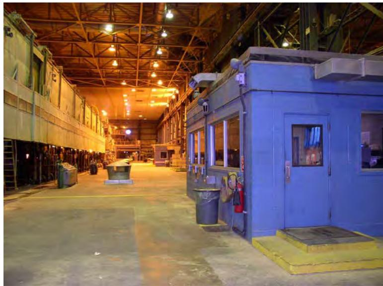
***Figure 4.30 - Acoustical control room and noise refuge in a paper manufacturing facility***
