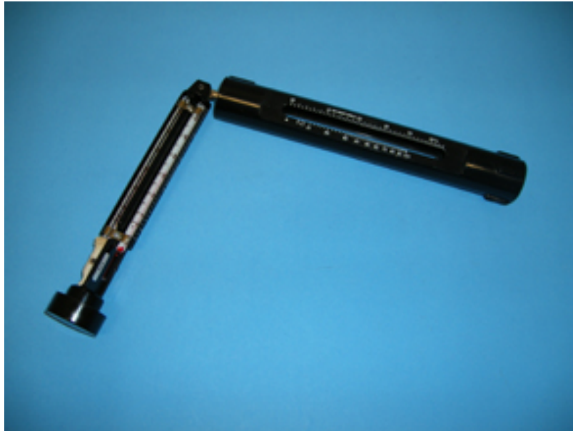
Figure 5.2 – Typical Sling Psychrometer
