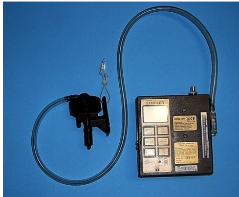
Figure 8.15 – Respirable Dust Sampling Train
