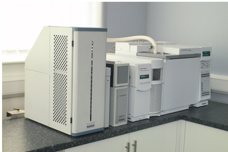
Figure 9.8– Thermal Desorption Unit with GC/MS
