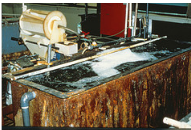
Figure 9.9 – Electroplating bath with detergent foam
