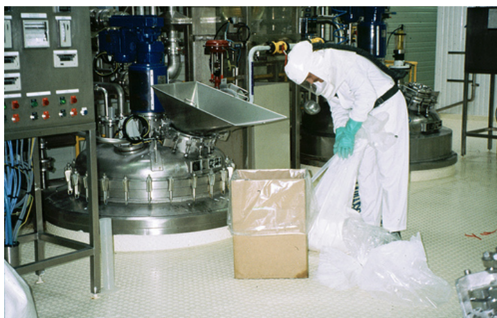
Figure 10.10 – Addition of sack of powder to reactor
