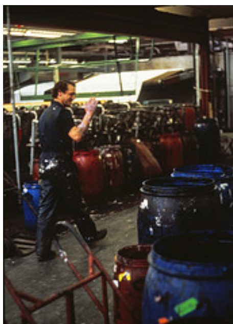
Figure 9.16 – Paint mixing – skin and airborne exposure can occur to solvents and pigments
