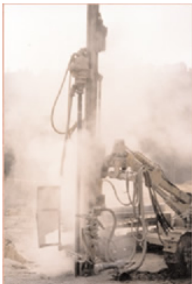
Figure 10.6 – Crawler mounted drill with no dust control
