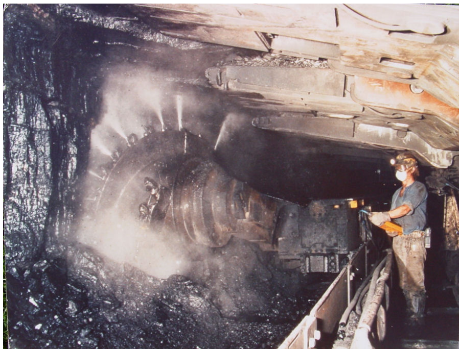
Figure 10.9 – Longwall coal mining with water sprays
