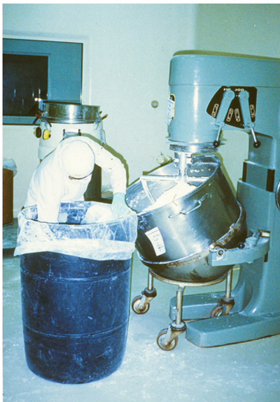
Figure 9.2 – Manual loading of open mixer from drum
