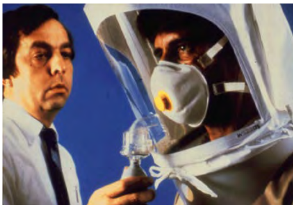
Figure 8.11 – Qualitative Fit Testing with Saccharin or Bitrex
