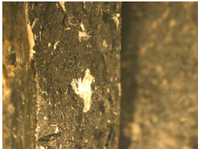
Figure 8.6 – Chrysotile fibres in asbestos cement
