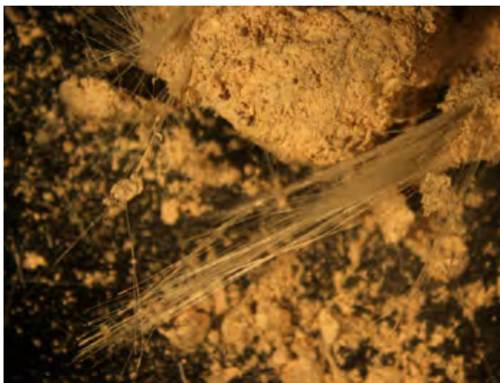
Figure 8.7 – Asbestos fibres in asbestos insulating board
