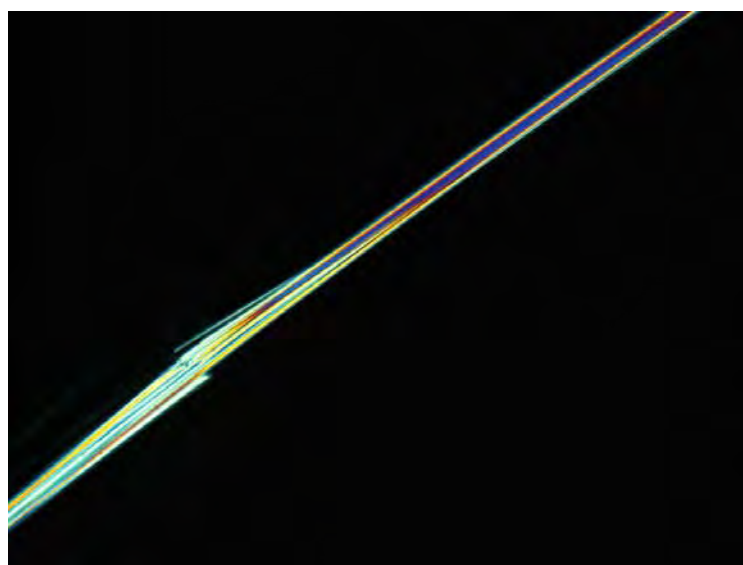
Figure 8.14 – Amosite fibres showing moderate birefringence
