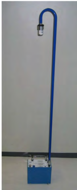
Figure 7.2 – High flow pump and sampling head
