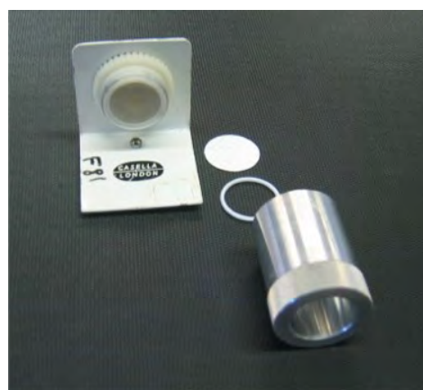
Figure 7.3b – Sampling head (exploded view)
