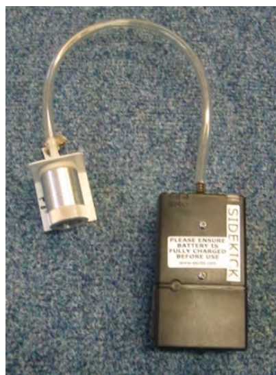
Figure 7.1 – Low flow pump and sampling head
