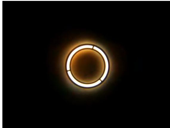
Figure 9.5 – Centring of phase rings (2)
