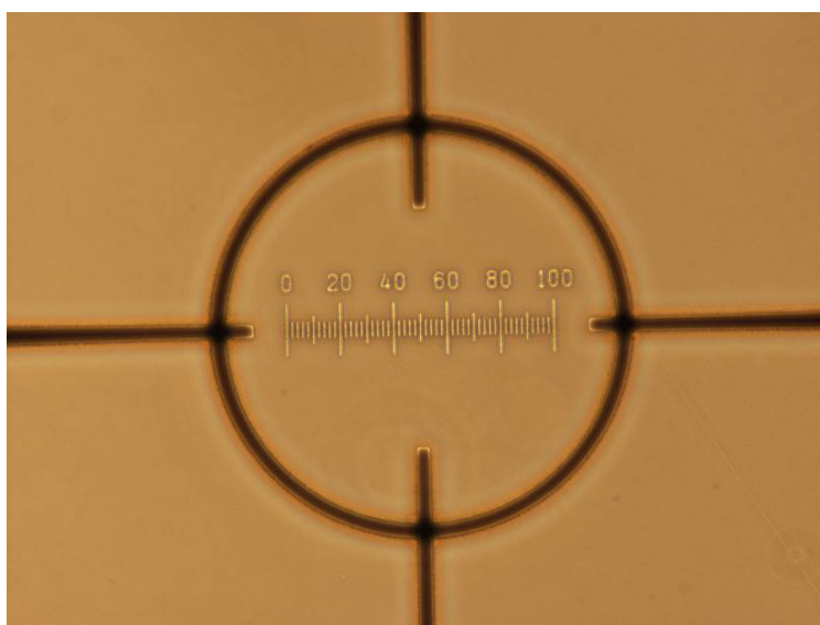
Figure 9.7 – Image of stage micrometer scale
