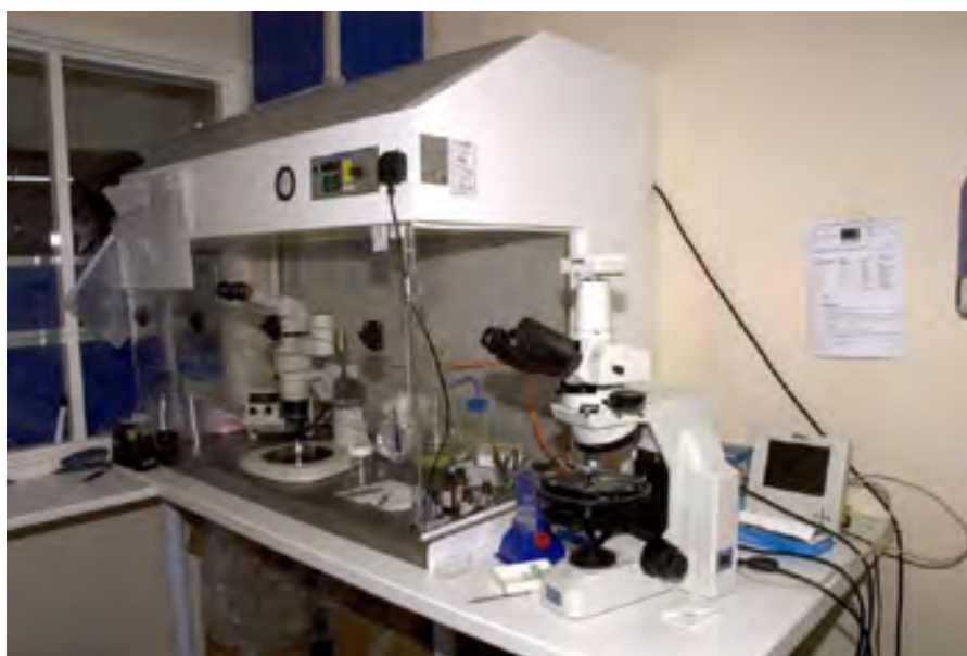
Figure 8.2 – Safety cabinet for asbestos bulk analysis
