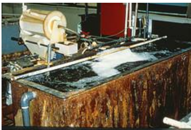
Figure 9.9 – Electroplating bath with detergent foam
