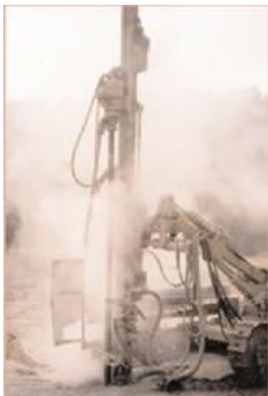
Figure 10.6 – Crawler mounted drill with no dust control
