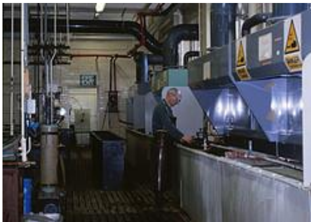
Figure 9.10 – Electroplating bath fitted with local exhaust ventilation
