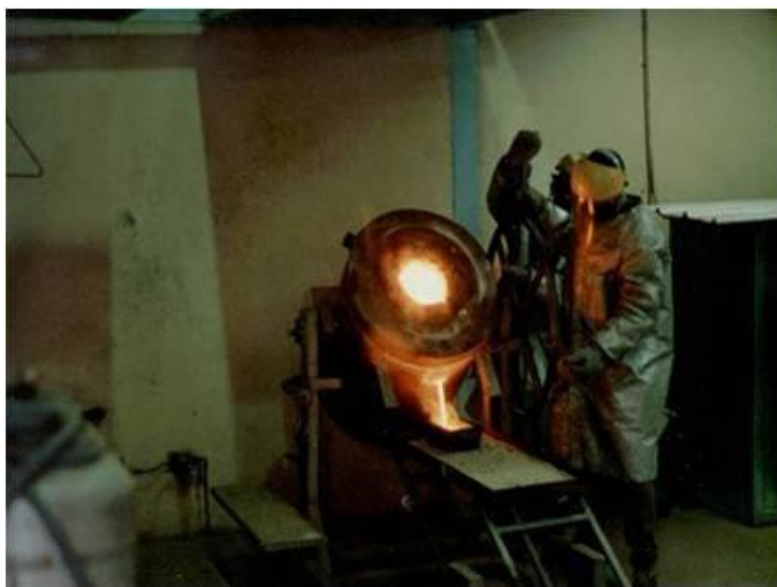
Figure 10.2 – Pouring molten gold
