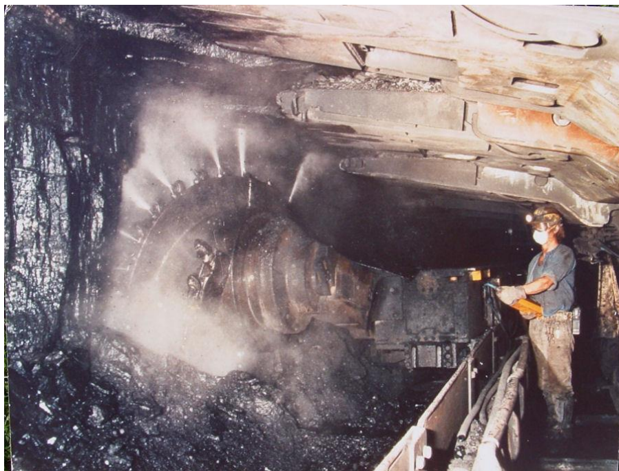
Figure 10.9 – Longwall coal mining with water sprays
