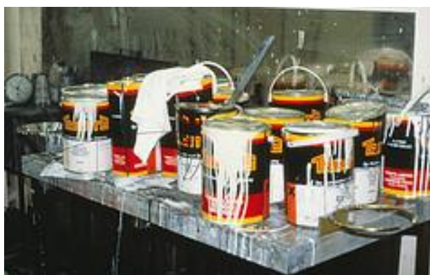
Figure 9.4 – Paint bench – open tins and rags soaked in thinners can be a source of exposure
