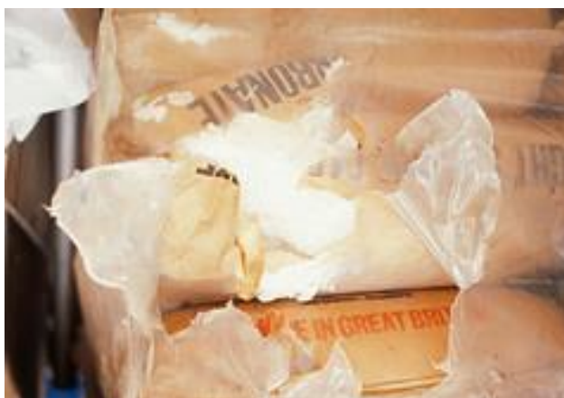
Figure 9.1 – Split bag containing sodium carbonate
