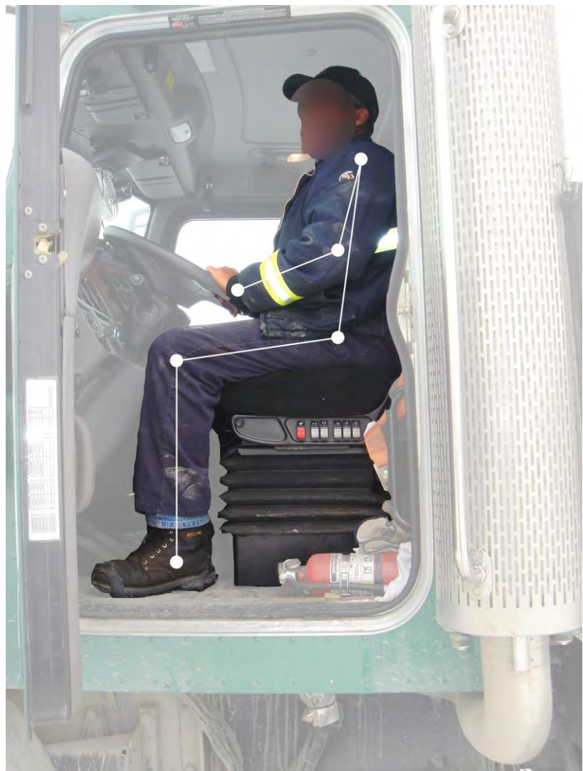
Figure 2.16 – Static Anthropometry of Seated Operator
