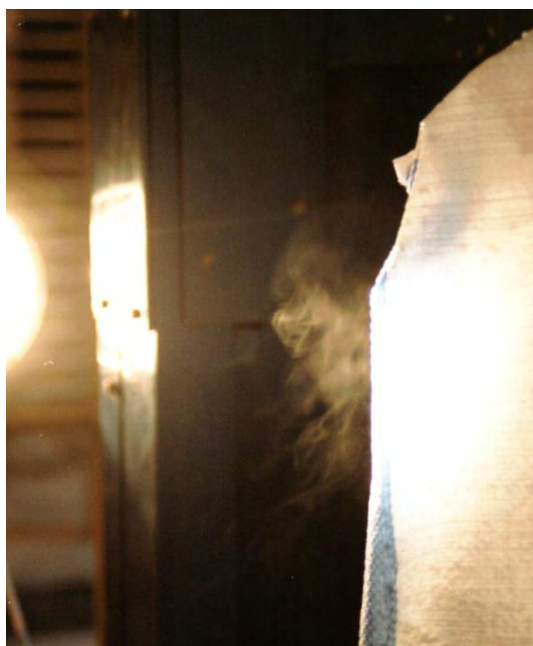
Figure 10.9 – Dust Lamp used to Highlight Fume Loss from Bags
