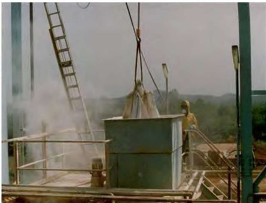
Figure 10.1 – Loading Hydrated Lime into Chute above Cyanide Mixing Tanks
