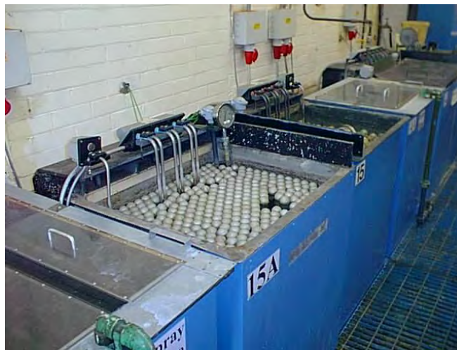
Figure 6.12 – A Plating Tank with Slot Extraction Along One Edge
