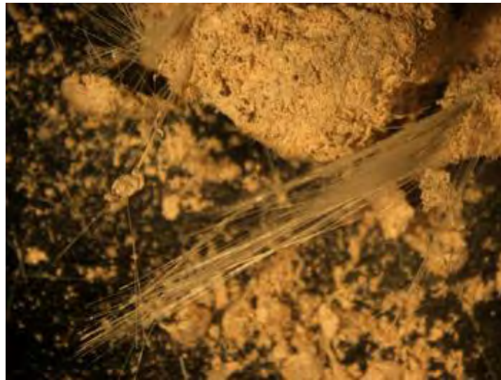
Figure 8.7 – Asbestos fibres in asbestos insulating board
