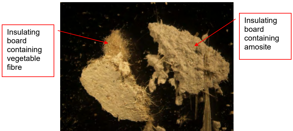
Figure 8.8 – Amosite fibres in asbestos insulating board next to insulating board containing vegetable fibres
