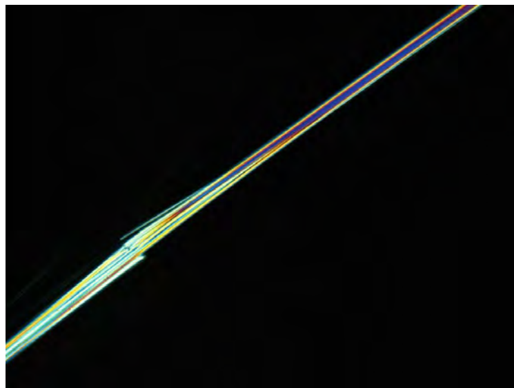
Figure 8.14 – Amosite fibres showing moderate birefringence
