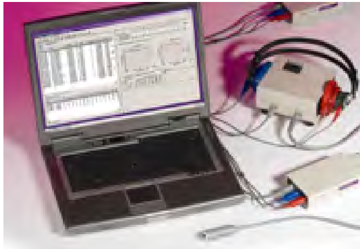
Figure 7.6 - Example of a computer-controlled audiometer. The audiometer functions are accessed with the computer keyboard
