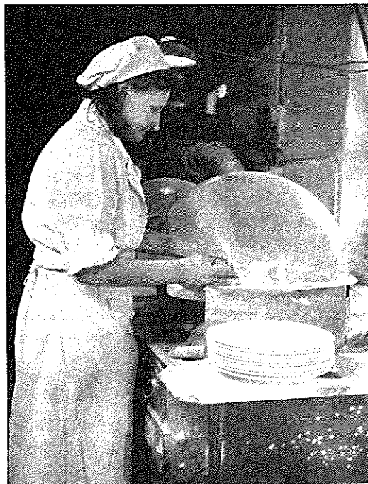
Figure 4.2. Two old hood designs (problems included: no physical separation of the workers breathing zones from the process; flatware and tools stored outside the hood; no air jet in hood to blow off residual dust. In the case of hood (a) the projected dust stream struck the workers midriff heavily contaminating her clothing and the perspex dome rapidly became scratched and difficult to see through).
