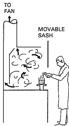
Figure 7.1 Examples of partial enclosures or receptor hoods.
