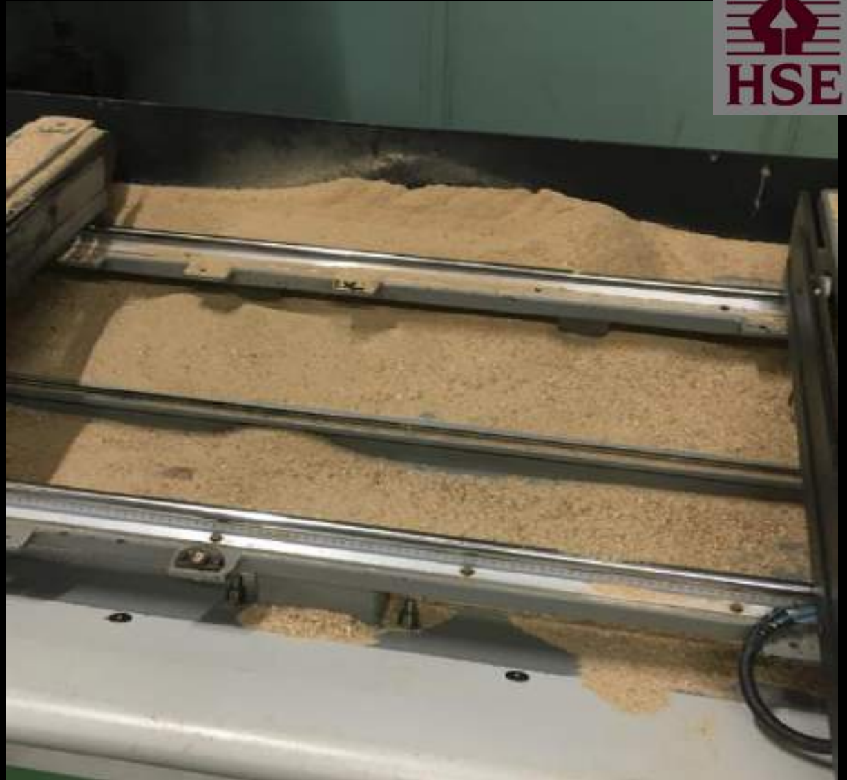
A machine with an LEV system that had just had a "thorough" examination
